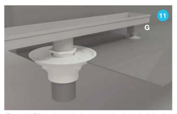
**Step 11.** Place the drain base into the threaded nipple **J**. Use the adjustable feet **G** to keep the drain channel into the correct position and level.
