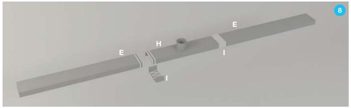
**Step 8.** Clean all parts. On a flat, stable surface, align the cut ends of the base with the outlet section. To join the base pieces **E** to the outlet **H**, attach joiner strips **I** to the underside of the seams, using clear PVC primer and PVC cement.
