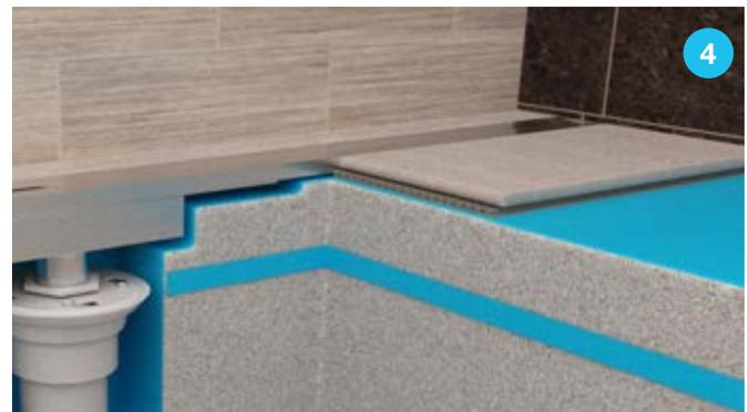
**Step 4.** Trowel mortar to required height.
