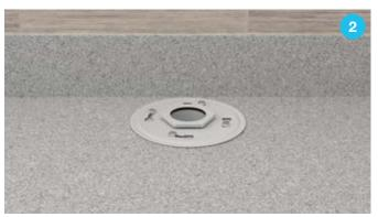
Step 2. Mark the center of your shower and screw threaded nipple into the drain flange, adjust to desired height.
